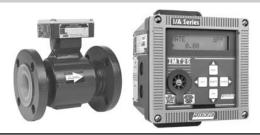
A Magnetic Flowmeter consisting of a flowtube, signal cable, and Transmitter measures flow rate of conductive liquids (usually water based) and transmits a proportional electrical signal.
