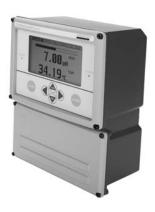
These Microprocessor-based, line-powered intelligent analyzers, when used with compatible Foxboro sensors, provide high accuracy measurement indication, output and alarming capability for pH, ORP, conductivity or resistivity. A human interface guides the user through intuitive, menu-driven configuration, calibration, status, and diagnostic procedures. A history log provides a report for up to 100 time and date stamped events.
