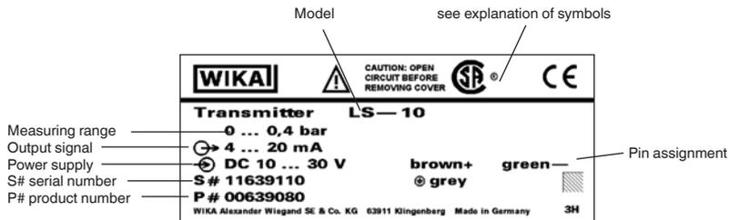
If the serial number becomes illegible due to mechanical damage or overpainting, traceability will no longer be possible.
