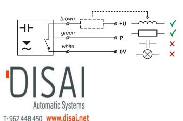
Note: In case of strong ambient electromagnetic interference, paralleling of conductors with power distribution, or for the distribution to distance over 30 m, we recommend to use shielded cable.
