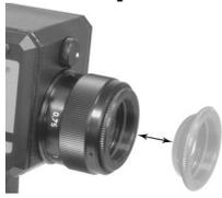
If using the close-up lens, the emissivity setting of the instrument (EMI) has to be corrected with the following factor (emissivity see **5.1**) due to reduced measuring signal:
