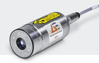
The Impac® IN 5 plus series infrared thermometers are specially designed for non-contact temperature measurements on non-metallic surfaces and also on painted, coated or anodized metals. These instruments are digital pyrometers equipped with a digital interface, enabling temperature indication and storage on a PC. A temperature sub range can be configured and the instrument parameters can be adjusted remotely.
