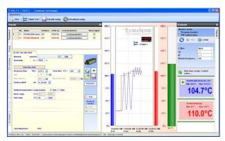
Measurement with Internal Temperature of radiation temperature and internal instrument temperature. Parameters can be changed during the measurement.
