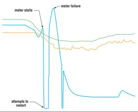
Note these actual lab tests. With gas in the process fluid, the competitor's meter goes into slug flow, stalls, tries to restart — but you get no reliable measurement while entrained gas lasts ...
