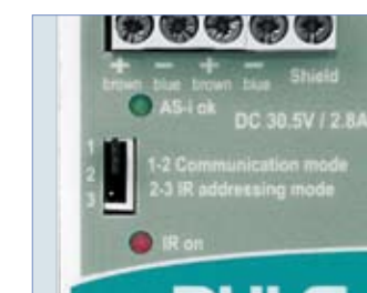
Easy commissioning: Supports addressing via infrared programming device.
