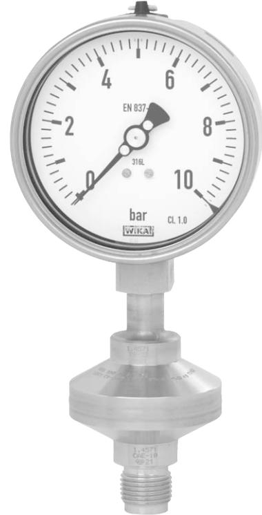
**Diaphragm Seal Model 990.34, Mb 52 mm process connection thread G ½ B (male), with Pressure Gauge Model 232.50 NS 100**
