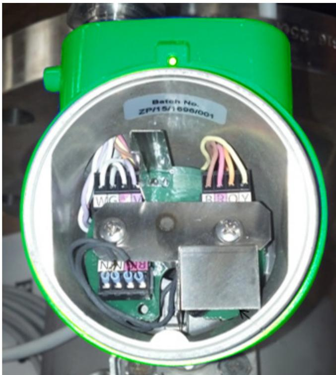
9. Replace the junction box cover. Rotate the set screw outwards from the junction box to lock the cover before operating the flowmeter.
