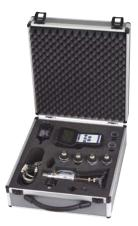
Calibration case, pneumatic; example with CPH6400
