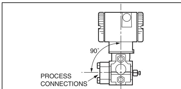
Figure 7. Vertical Mounting Showing Process Connections at 90 degrees
