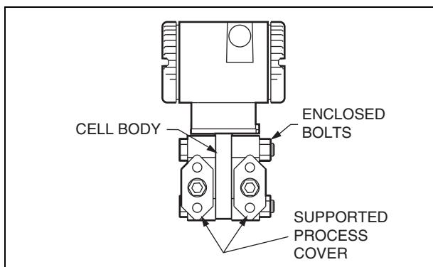
Figure 6. Biplanar Construction
