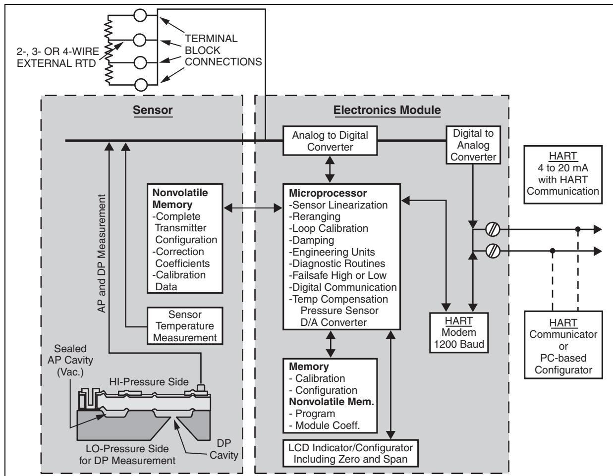
Figure 16. IMV31 Functional Block Diagram for HART Communication
