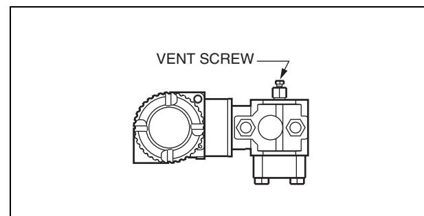
Figure 9. Horizontal Mounting - Cavity Venting and Self-Draining into Process Line
