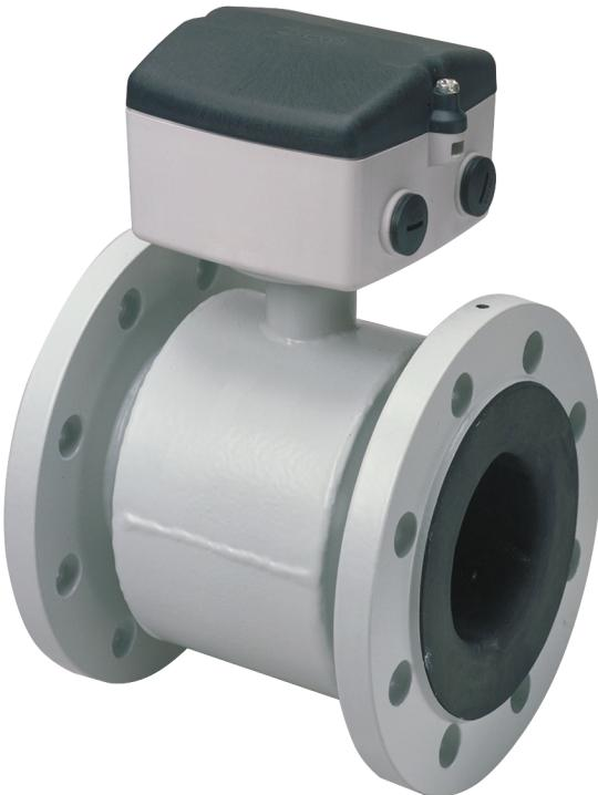
The Foxboro® brand 9100A Series Magnetic Flowtube together with an IMT25 or IMT25L Magnetic Flow Transmitter, combine to form a Magnetic Flowmeter with pulsed dc excitation. It is designed for use with conductive fluids in general purpose, and waste and water applications. The transmitter converts the low level, high impedance signal from the lined flowtube to a scaled transmission signal, either 4 to 20 mA, digital, or pulse output, that is proportional to volumetric flow rate.
