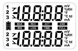
°C.. Temperature in degrees Celsius °F.. Temperature in degrees Fahrenheit %RH....... Relative humidity (KH 250) td.. Dew point temperature (KH 250) V or mV Voltage expressed in V or mV A or mA Current expressed in A or mA
