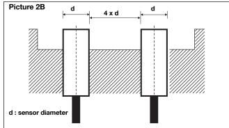
For sensors installed opposite each other, a minimum space of 6 x Sn (the nominal sensing distance) must be observed (See Picture 3).
