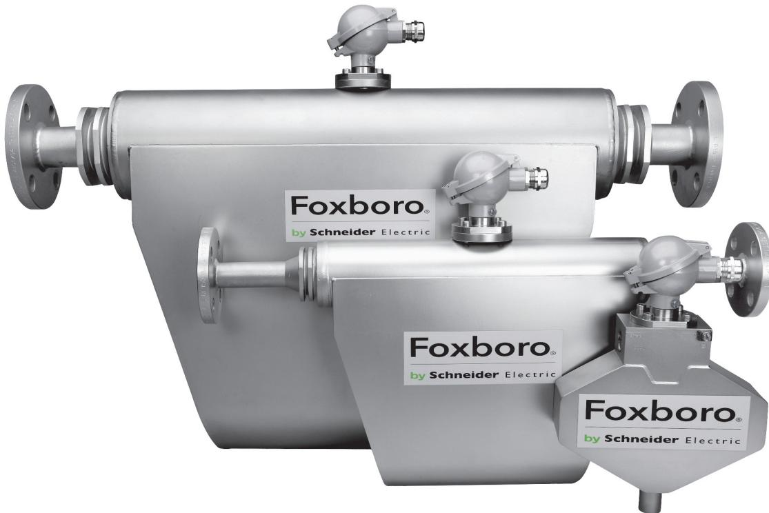
*Foxboro® brand CFS25 Coriolis flowtubes combine with a Model CFT51 Digital Coriolis Mass Flow Transmitter to form an I/A Series® Coriolis Mass Flow and Density Meter. The principle of Coriolis acceleration is used, which allows true mass flow rate measurements of fluids to be made directly without the need for external temperature, pressure, or specific gravity measurements.*
