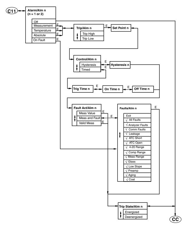
Figure A-12. Configure Alarm Structure
