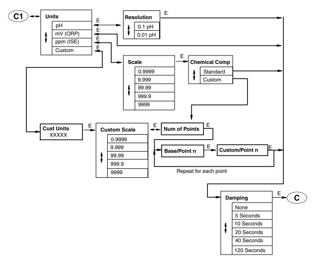
Figure A-2. Configure Measurement Structure
