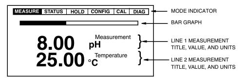
Figure 14. Sample Dual Measurement Screen
