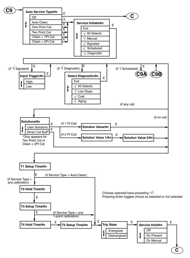
Figure A-9. Configure Auto Service Structure
