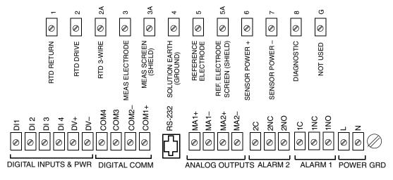
Figure 7. Wiring Connections for 875PH Analyzer
