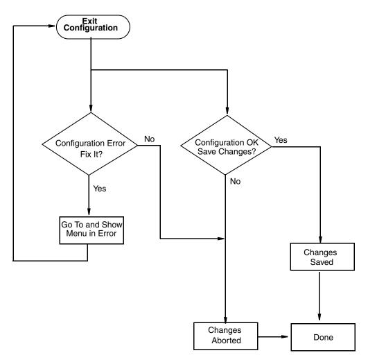
Figure 30. Configuration Mode Exit Flow
