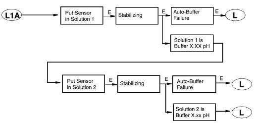
Figure 26. Smart Calibration Structure Diagram
