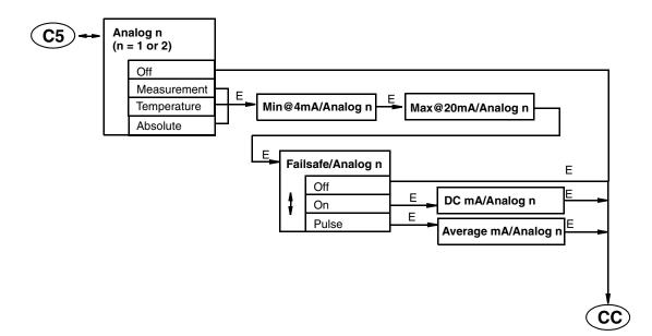
Figure A-6. Configure Analog Structure
