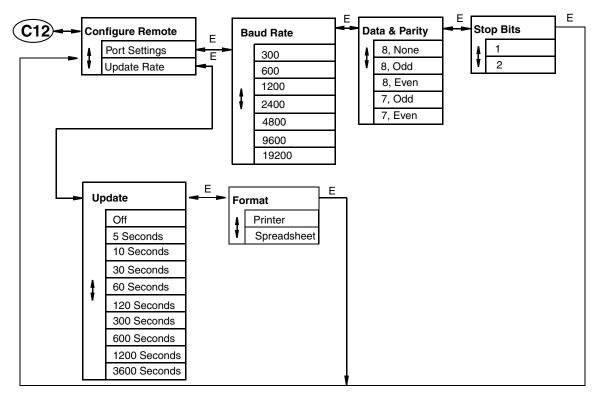
Figure A-13. Configure Remote Structure
