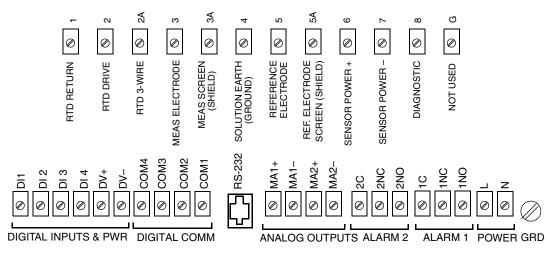
Figure 1. Wiring Connections (Style B)
