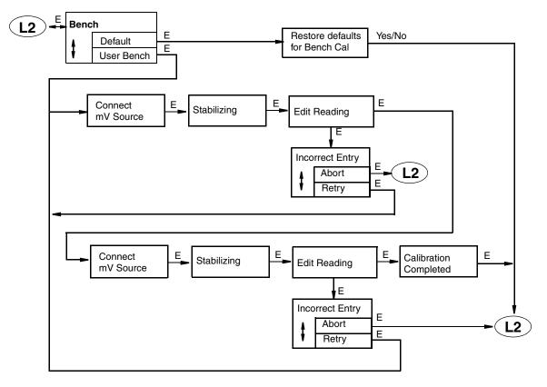
Figure 27. Bench Calibration Structure Diagram
