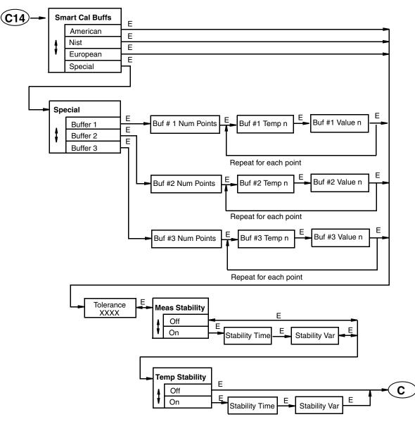
Figure A-15. Configure Cal Parameters Structure
