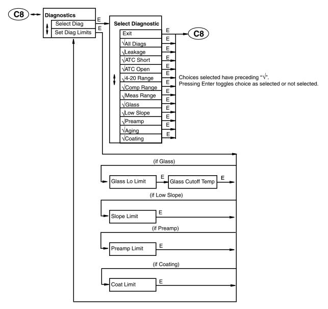
Figure A-8. Configure Diagnostics Structure
