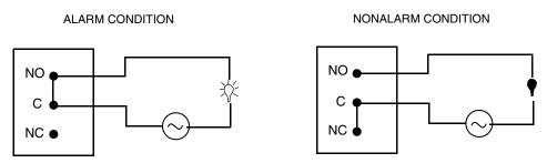
Figure 11. Alarm Wiring in Energized Trip State
