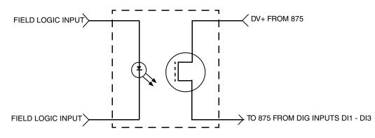
Figure 9. Optical Isolated Analog Switch
