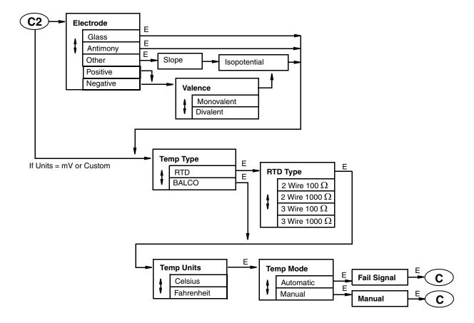
Figure A-3. Configure Sensor Structure
