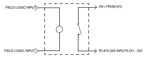
Figure 10. Electromechanical Relay Interface
