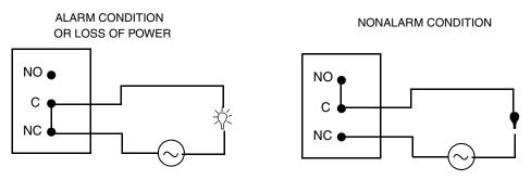
Figure 12. Alarm Wiring in De-energized Trip State
