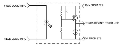
Figure 8. Optically Isolated Interface 24 V dc, FET Output PLC
