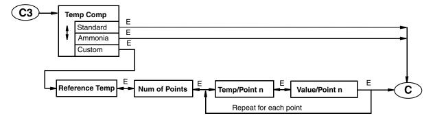
Figure A-4. Configure Tempcomp Structure
