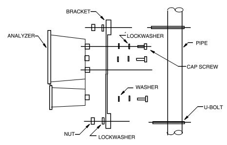
Figure 6. Pipe Mounting (Vertical Pipe Mounting Shown)
