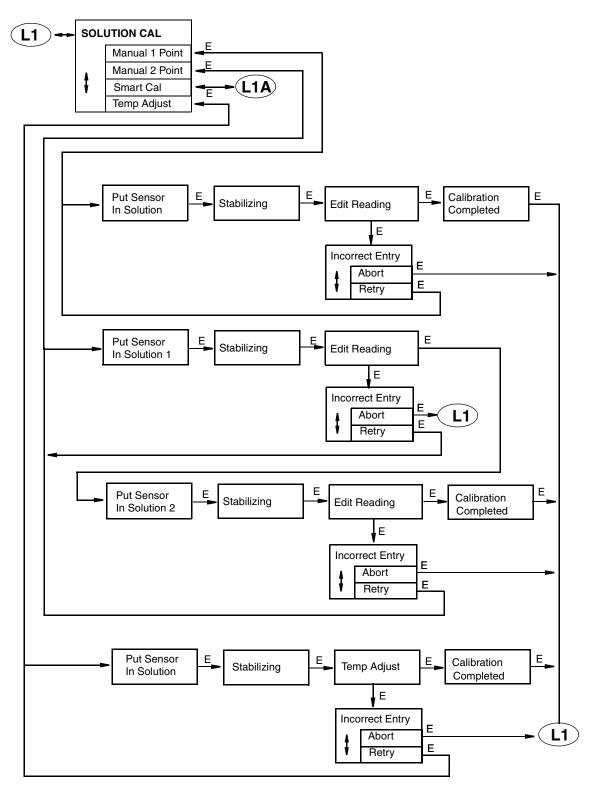
Figure 25. Solution Calibration Structure Diagram
