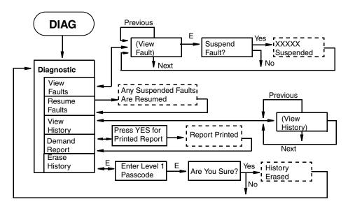
Figure 35. Top Level Diagnostic Mode Structure
