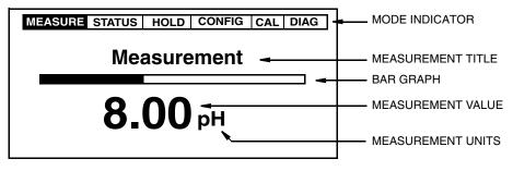
Figure 15. Sample Single Measurement Screen
