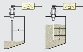
Measurement of electrically non-conductive materials: The capacitor is made by electrode of the sensor and the wall. The dielectric is done by air or the material.
