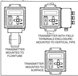
Figure 1. Multiple Packaging Configurations
