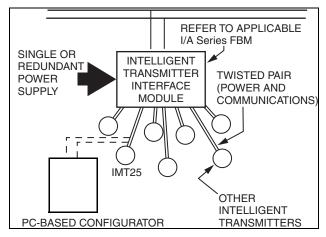
Figure 5. Functional Block Diagram FoxCom Digital Output Only
