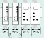
$\begin{array}{ll} \mbox{Dimensions} & : 22.5 \mbox{x} 75 \mbox{x} 120 \mbox{ mm} \\ \mbox{With } \mu \mbox{console} & : 26.5 \mbox{x} 80 \mbox{x} 130 \mbox{ mm} \end{array}$
