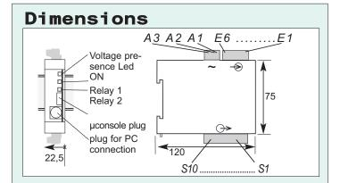
Case : (H x L x D) 75 x 22,5 x 120 mm with μconsole : 80 x 26,5 x 130 mm Self-extinguishing case of black UL 94VO ABS. For mounting in electrical switchbox : latching on symmetrical DIN rail. *Consult with us for rack versions.*
