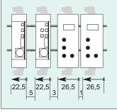
To insert the µconsole : mount the instruments vertically (on horizontal DIN rail) and provide a 5mm spacement.
