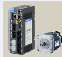
Closed loop stepping systems provide the ease of use of stepping systems and the reliability of servo systems. The stepping motor in these systems has an encoder that provides feedback to the driver to prevent step-out (misalignment), which is a weak point of stepping motors.
