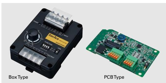
You can control the speed of fans with the PWM control function. Contributes to reduced system power consumption and noise.
