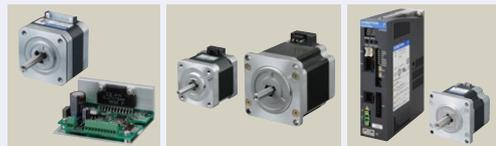
Stepping motors are driven precisely at a set angle (basic step angle) according to the number of pulses input to the driver from a pulse oscillator. These use open-loop control without an encoder (position detection sensor), helping build simple and low-cost systems. Ease of use is a key point. In addition, they use holding force when stopped, and feature stable stopping without micro vibrations.
