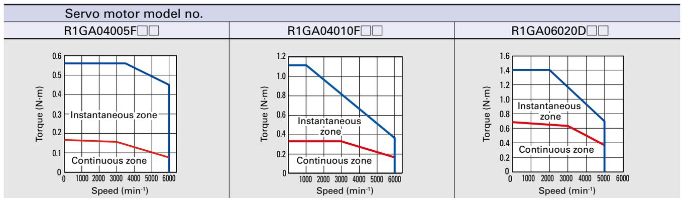
Note 1: The characteristics curves above are for when a 48VDC main circuit power supply is used and the length of the wiring between the servo amplifier and servo motor is 2 m.
