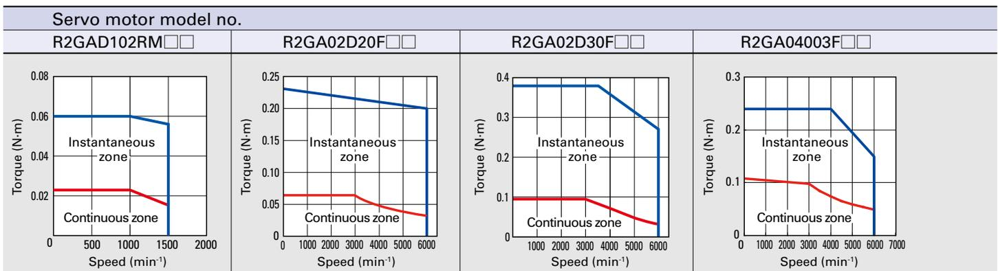
Note 1: The characteristics curves above are for when a 48 VDC main circuit power supply is used and the length of the wiring between the servo amplifier and servo motor is 2 m.
