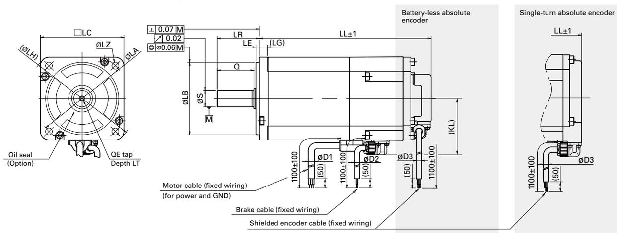
This drawing is for a motor equipped with a brake.
