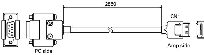
Connect to a PC with an RS-232C serial cable
