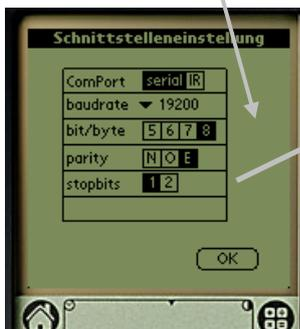
In order to programme parameters for the FR85ILLG via the serial connection, the following interface parameter must be set!
