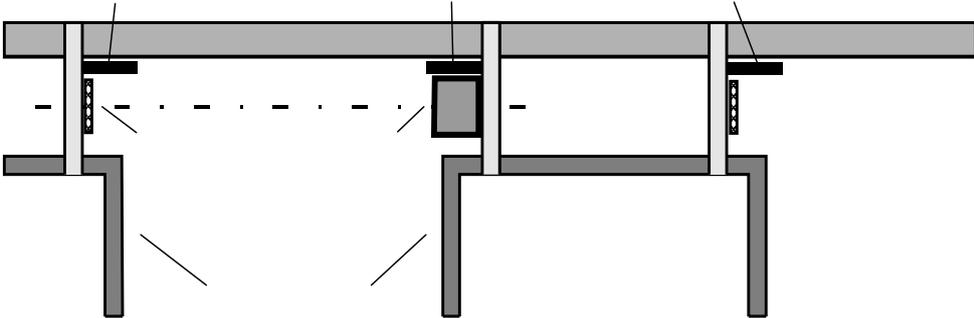
The illustrated frame protection prevents damage occurring to sensors and reflectors when the EMS vehicles are pushed up close together during service interventions.
