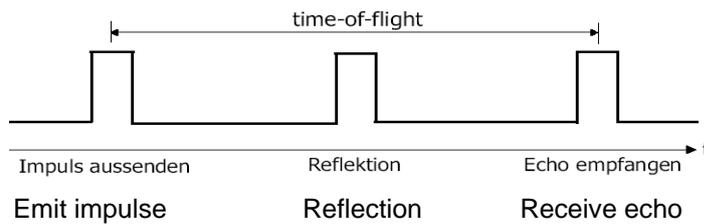
Use of this physical principle makes RailPilot ideal for optical anti-collision distance measurement.
