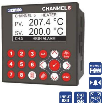
8 x Pt-100 inputs, different SET values for each channels, Relay or Transistor Alarm outputs for each channels, Low, High and Range alarms for each channels, Data logging by USB memory, Networking between multiple devices by RS-485 serial communication.
