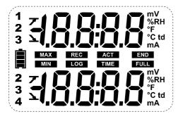
°C.. Temperature in degrees Celsius °F.. Temperature in degrees Fahrenheit %RH..... Relative humidity (KTH 350) td.. Dew point temperature (KTH 350)
