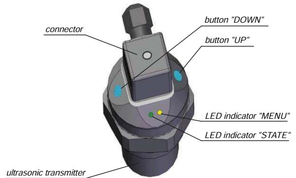
Full view of ultrasonic level meter
