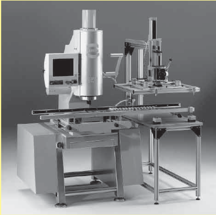
Fig. 11: Bestseller CPM prestige with insertion removal station , adaptable to all HARTING press-in machines.
