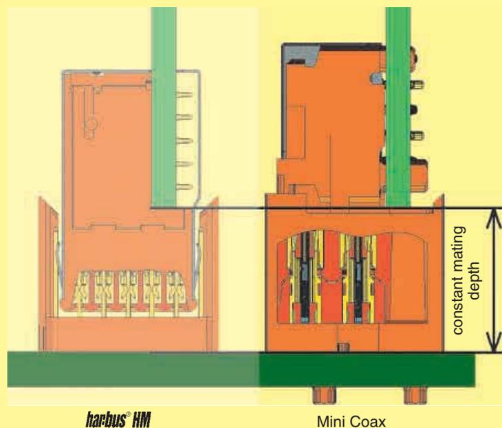
Fig. 2: Cross section of both connector types
