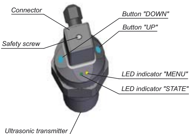
Fig. 16: Full view of ultrasonic level meter
