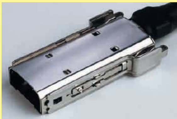
Fig. 2: 360° screened-can construction with locking levers
