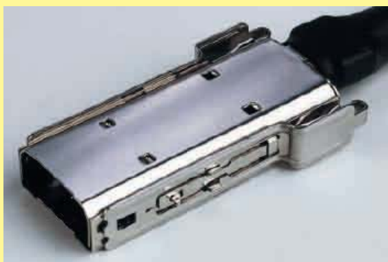
Fig. 2: 360° screened-can construction with locking levers
