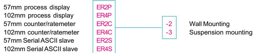
For example model ER4P-2 is a wall mounting 102mm process display
