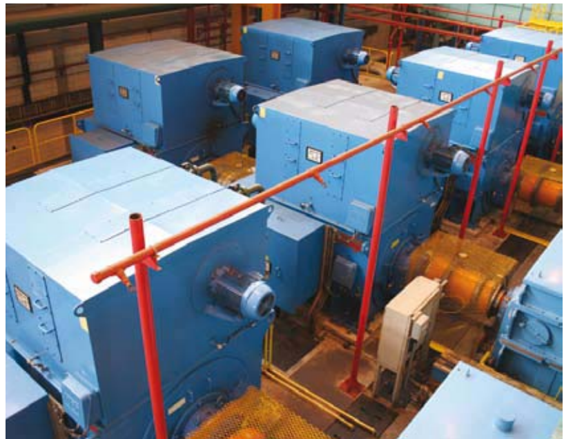
Synchronous Motors SDL800, 3000 kW, 3100 V. Application: Laminating machines (steel plants).
