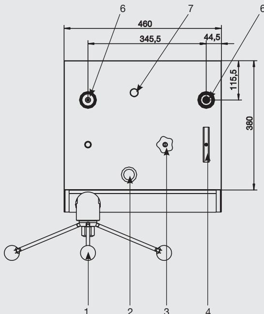
The dimensions of all 3 pump models are identical.
