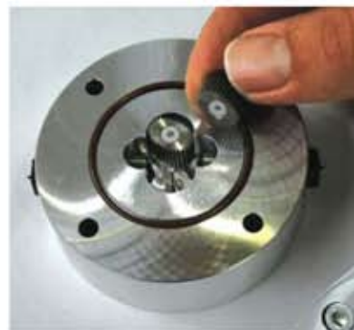
Two oval shaped gears (rotors) are the only moving parts within the measuring chamber
